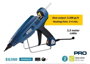
Industrial glue gun with an exceptionally high glue output of 2,200 g/hour. Designed for demanding use. Convenient adjustable temperature (120-230 °C) for versatility and working with different materials and ergonomic 4-finger trigger to reduce fatigue.
